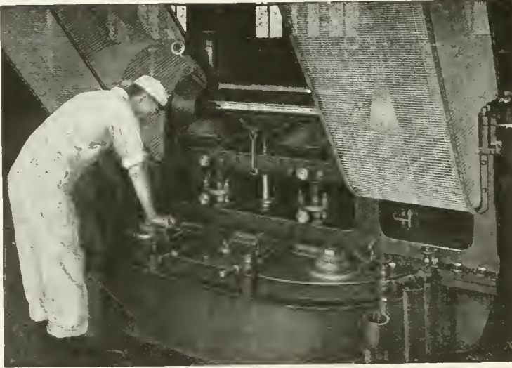
The solid ingredients of oleomargarin are melted, mixed with the liquid oils, and churned together with milk. Later the surplus moisture is removed, and the small granules of the product are worked into a complete and plastic mass.
